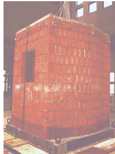
Figure 18: Cored brick masonry
