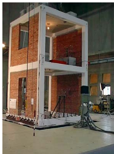
Figure 15: RC frame with masonry infills
