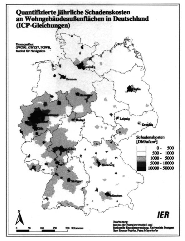
*Fig. 7: Quantified annual cost of damage to buildings due to atmospheric corrosion in Germany given as DEM/year/km*<sup>2</sup>
