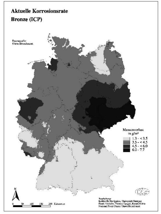
*Fig. 6: Map of the annual corrosion rate of bronze in Germany in the years 1993-95 based on doseresponse functions from the UN ECE Material Exposure Programme*
