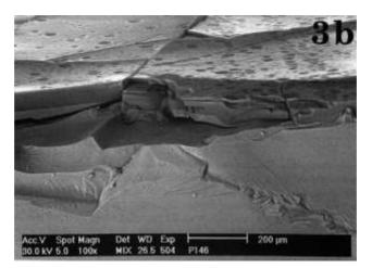
*Fig. 4: Scanning electrone micrograph of an edge of a corroded glass, showing the corrosion and silicagel layer on top of the bulk glass.*
