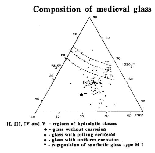
Fig. 3: Composition of medieval glass represented in a triangular diagramme and ist stability against acid attack (hydrolitic classes)
