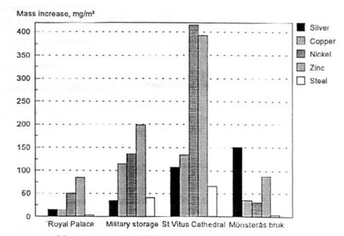
Mass increases for different metals after one year exposure at the different test sites.
