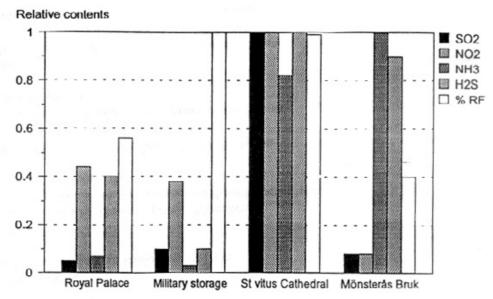
Relative concentrations of gases and relative humidity measured at the different test sites.
