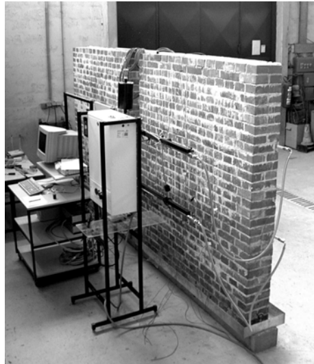
Figure 19. Laboratory testing of wall tempering performance.
