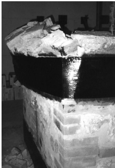
FIGURE 5: The containing action of FRP sheet
