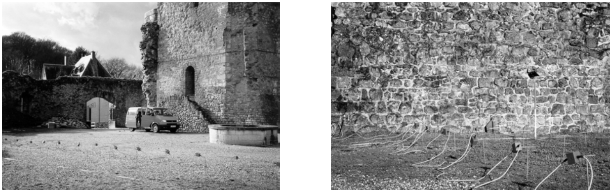
Fig. 3: Electrical resistivity tomography (ERT) at the medieval castle of Useldingen (Luxembourg), field display with multi-electrode array RESECS.
