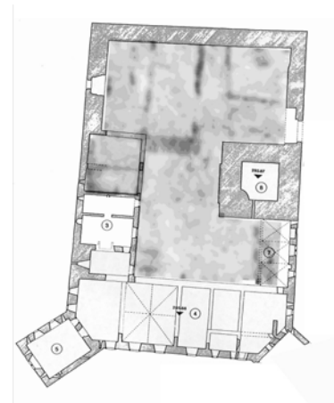
Fig.5: Left: Ground Penetrating Radar (GPR), field display, right: GPR horizontal depth slice showing hidden building structures (medieval castle of Koerich, Luxembourg)
