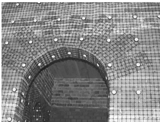
Fig. 16 – Reinforced test specimen
